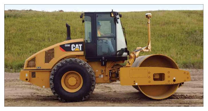
**GPS Mapping and Measurement.** Senses soil compaction as it works and correlates the data with the GPS position of the measurement. These capabilities improve work quality while lowering owning and operating costs, reducing necessary manpower, and optimizing productivity.
