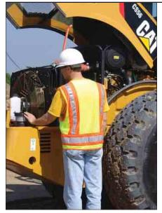
The one-piece fiberglass hood tilts forward for exceptional access to the engine and cooling system. Daily service points are accessible from ground level and are grouped on one side of the machine.
